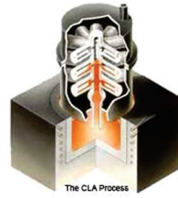
The "CLA" counter gravity investment casting process, (© Hitchiner Manufacturing Co., Inc.)
